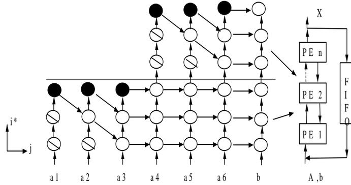
Fig.3.9. Partitioning of the Jordan –Gauss DG
