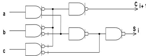
Fig. 4.10. The 6-th gates version of the one-bit adder
