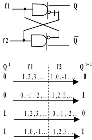
Fig. 4.20. Current-mode flip-flop circuit and its operations
