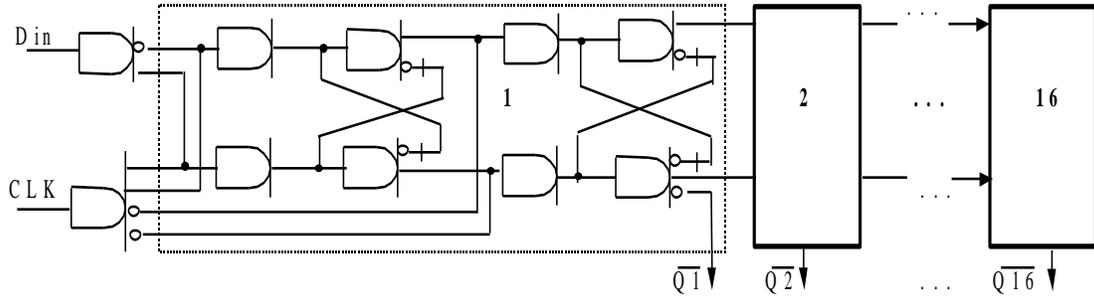
Fig. 4.23. Current-mode 16-cells one-bit FIFO circuit – base of the LUT  $F'$  and  $G'$
