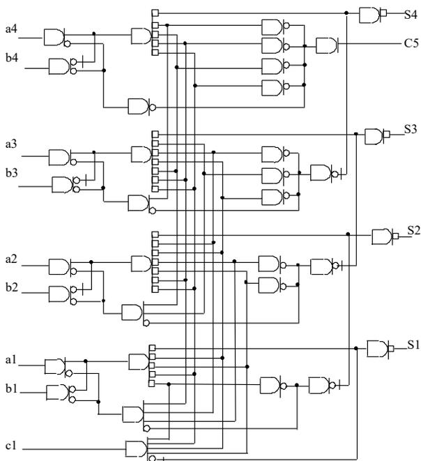
Fig.4.12. Fast 4-bit adder with the parallel propagation of the carry out bit
