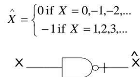
Fig.4.3. Current-mode anti-inverter
