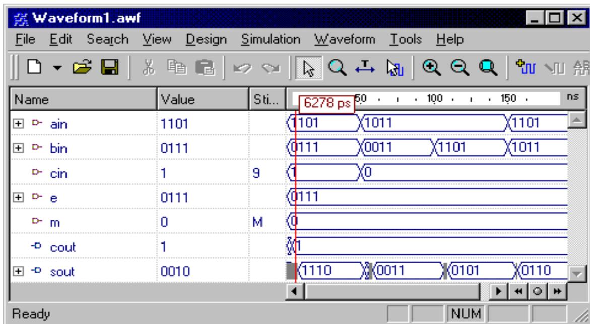
Fig.4.15. Results of simulations of designed current – mode ALU 74S181( $m=0$ ;  $e=1110$ ).
