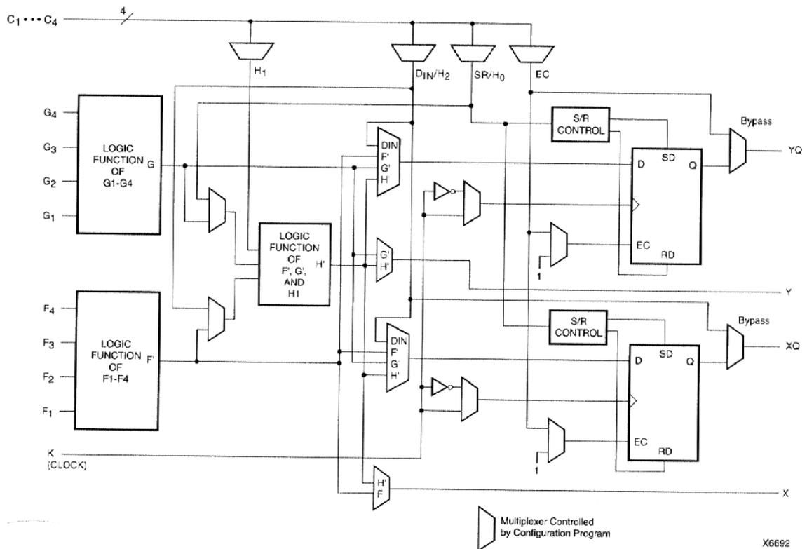
Fig 4.18. Simplified block diagram of XC4000 series CLB
