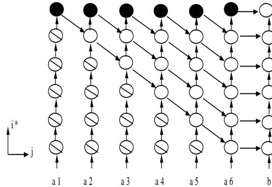
Fig.3.6. Transformation of Jordan Gauss algorithm DG
