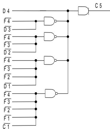
Fig.4.11. Realization of the parallel propagation of the carry bit  $C_{i+1}$
