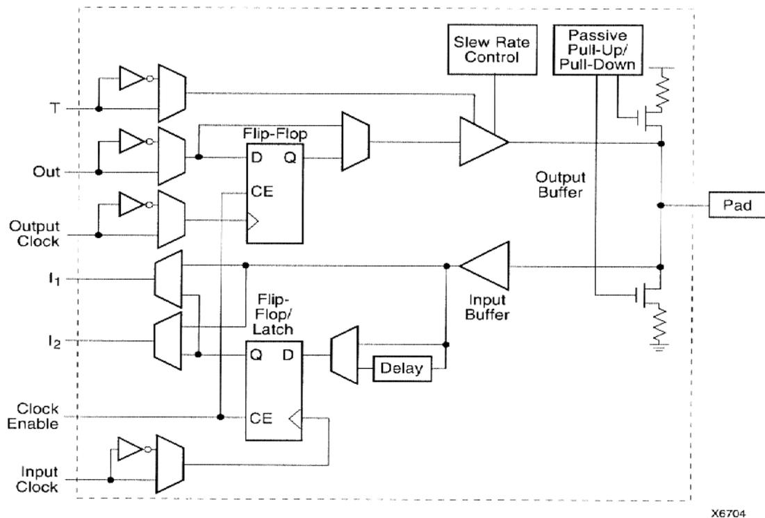
Fig 4.17. Simplified block diagram of XC4000 series IOB
