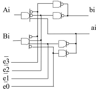
Fig. 4.14. The structure of the first cascade of the ALU 74S181.
