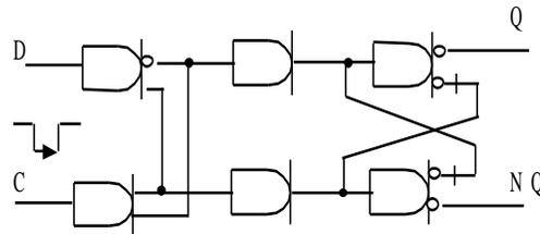
*Fig. 4.21. Current-mode low level sensitive D-trigger*
