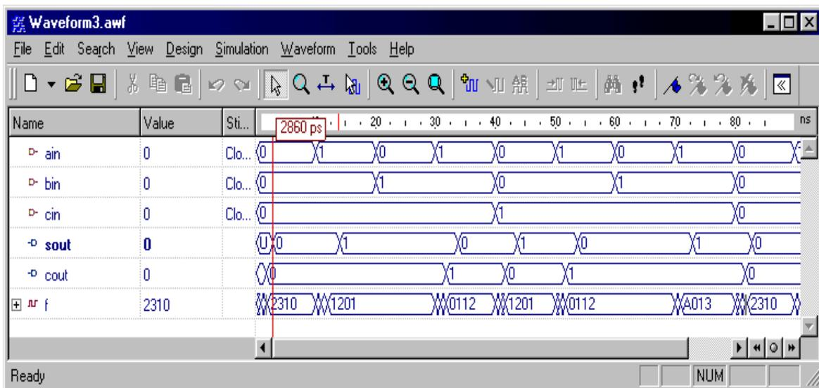
Fig.4.13. Results of simulation of designed one-bit current – mode adder.
