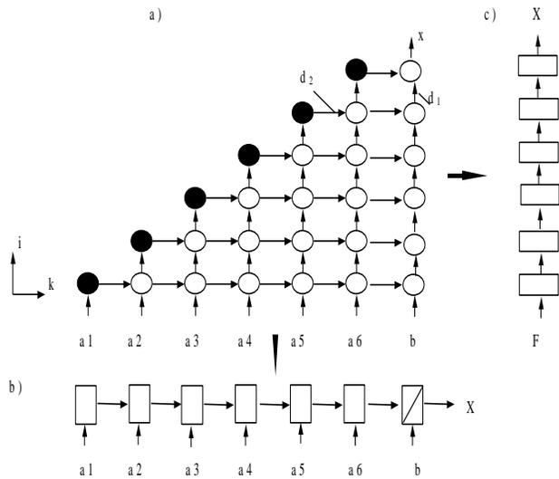
Fig.3.5. 2-D DG of Jordan-Gauss algorithm and 1-D architectures of processor arrays
