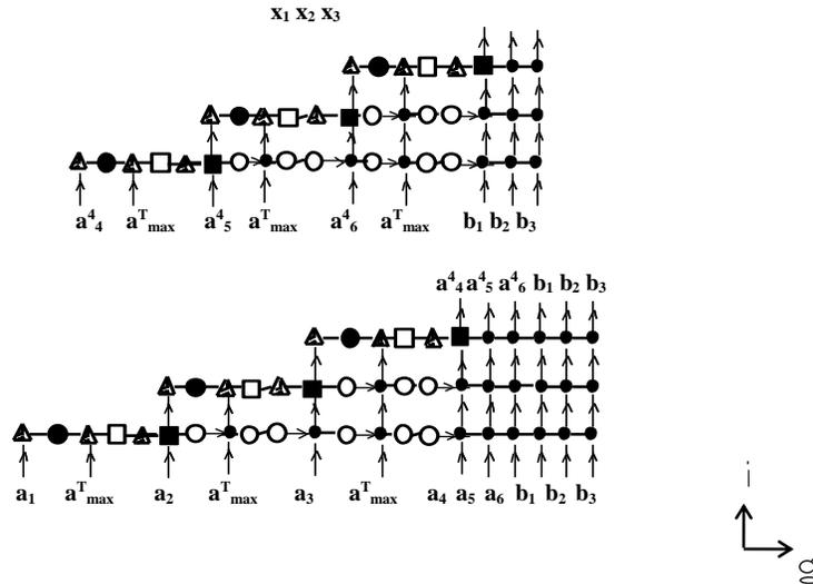
Fig.3.11 Partitioning of the fault-tolerant Jordan-Gauss algorithm
