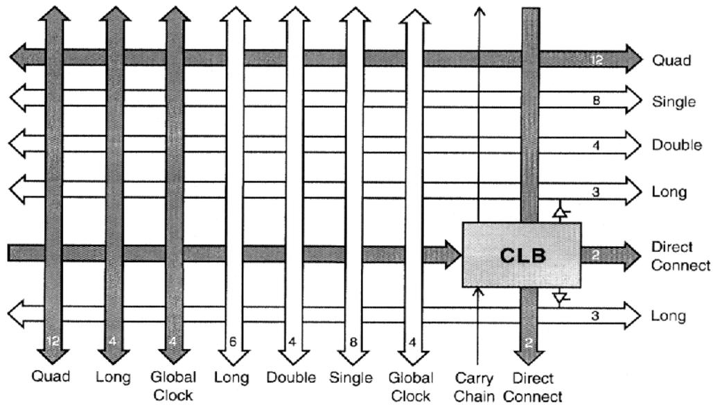
Fig 4.16. Simplified block diagram of FPGA XC4000 series cell
