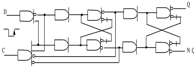
*Fig. 4.22. Current-mode rising clock edge driven D-trigger*
