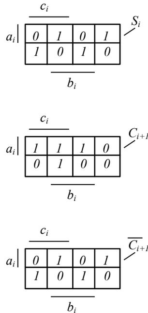
Fig.4.4. Vetch - Karnaugh's diagrams of the functions  $s_i$  and  $c_{i+1}$ .
