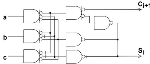
Fig. 4.5. The 7-th gates version of the one-bit adder
