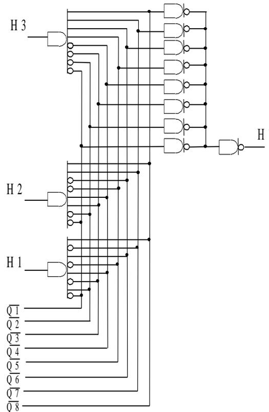
Fig. 4.24. Current-mode prototype of the LUT  $H'$  multiplexer circuit
