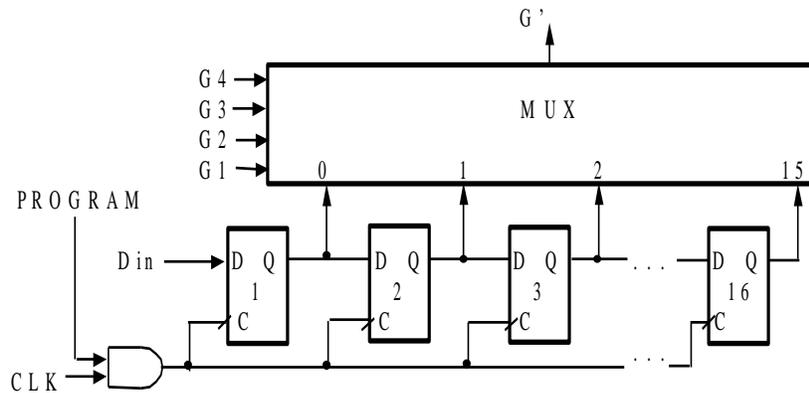
Fig. 4.19. Example of the internal structure of 4-inputs LUT (function generator  $G$ )
