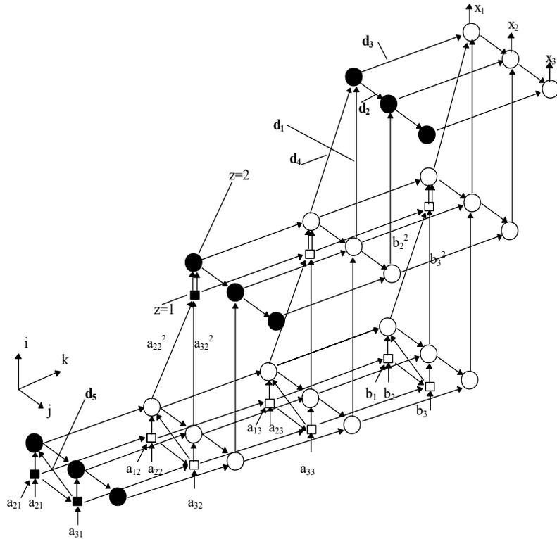
Fig.3.4. Basic dependence graph of Jordan-Gauss algorithm
