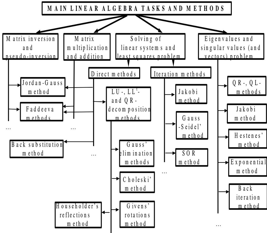
Fig.1.1. Main linear algebra tasks and methods
