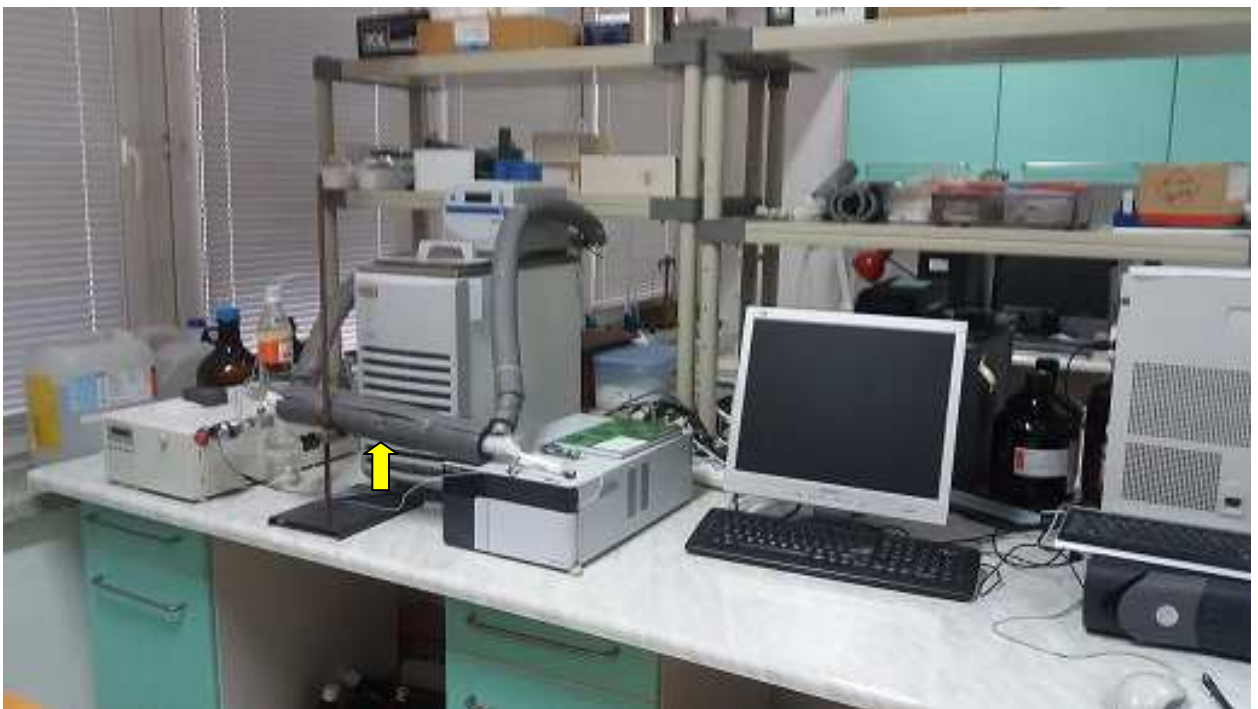
FIGURE 7. Temperature controlled inclusion chromatography: hardware setup for HPLC-DAD system. Yellow arrow indicate insulated water jacket containing HPLC column equilibrated with cyclodextrin modified mobile phase.
