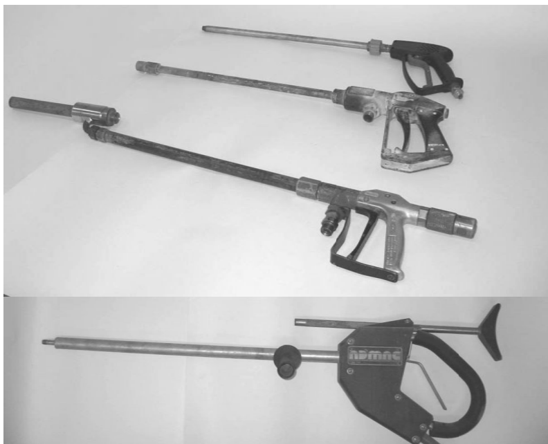
Fig. 3. Examples of high-pressure guns of lance type made by Woma and NDMNC manufacturers
