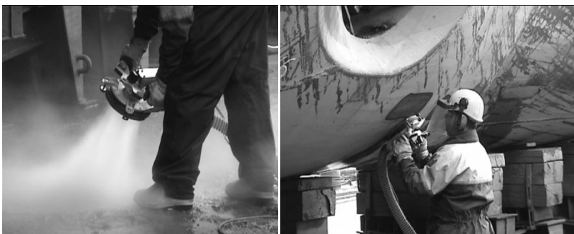
Fig. 13. Application of high-pressure manual working head Hand Held AQUABLAST type FRWV 3000
