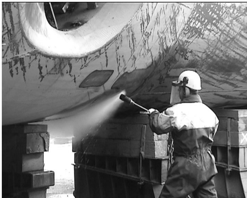
Fig. 11. Application of high-pressure gun equipped with super fast rotary RD 3000 type working head made by Hammelmann that includes magneto-dynamic brake
