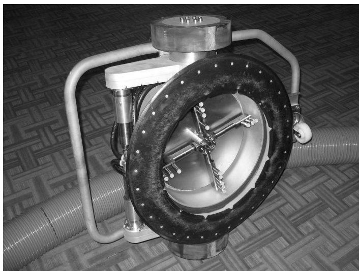
Fig. 17. View of SpiderJet 3000 inside showing rotor with nozzles and suction gasket (on the first stage)
