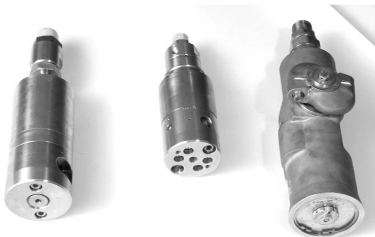
Fig. 7. Examples of high-pressure slow motion rotary working heads equipped with its regulation systems type RD 1500 (left), RDM 250 (center) and Aquamat XL 1500-2 (right)
