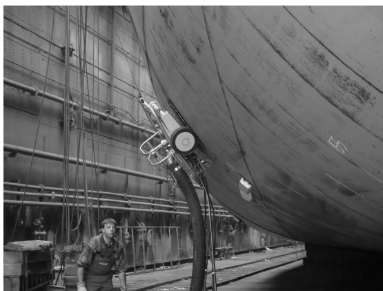
Fig. 15. SpiderJet during ship's hull cleaning in "GRYFIA" shipyard
