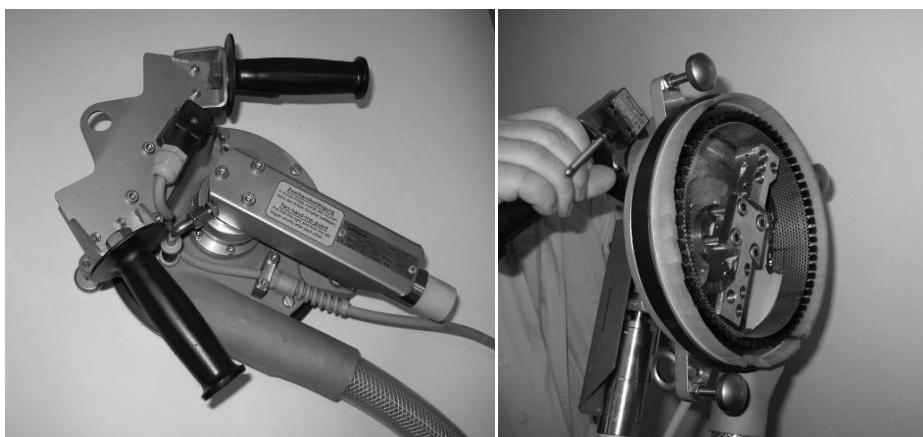
Fig. 1. Example of manual cleaning units using high-pressure water jet Aquablast® Hand Held type FRWV 3000
