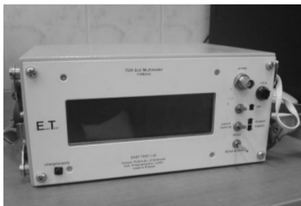
Fig. 7. Mobile TDR Multimeter (FOM – Field Operated Multimeter) applied in the presented in-situ experiments
