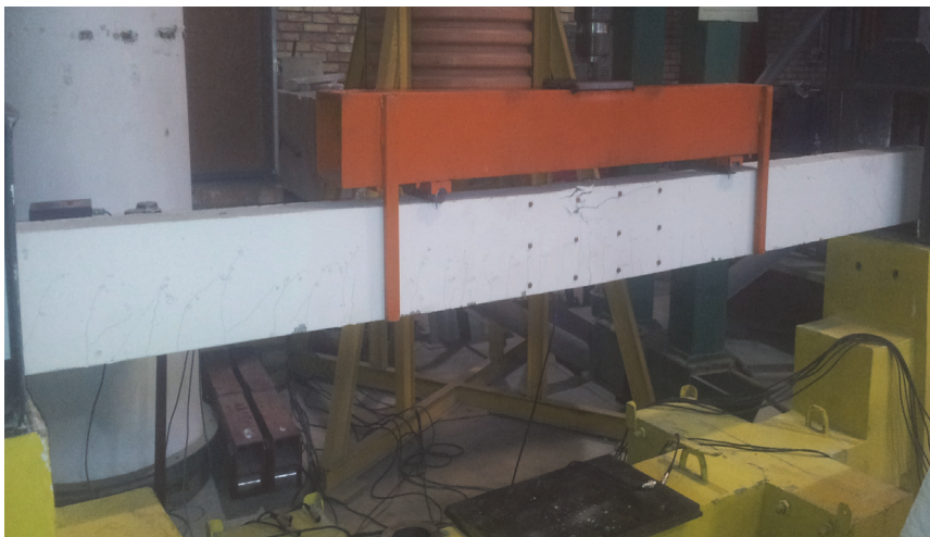
Fig. 2. The view of tested large scale beam made of RAC
