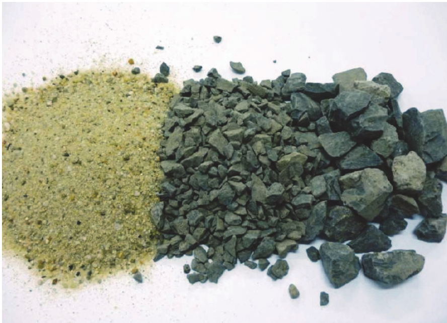
Fig. 1. Aggregates used in the research programme (photo by T. Ponikiewski) (from left: natural sand 0–2 mm, crushed basalt 2–8 mm, crushed basalt 8–16 mm)
