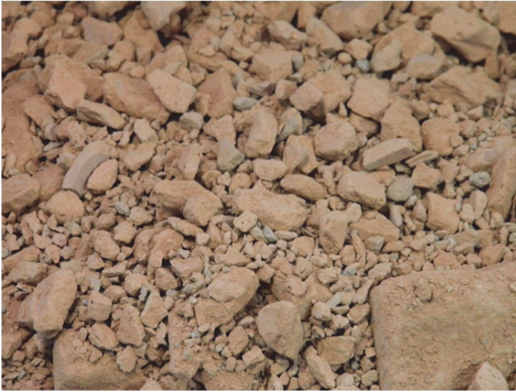
Fig. 2.3. Ground ceramic waste used as coarse aggregate[11]
