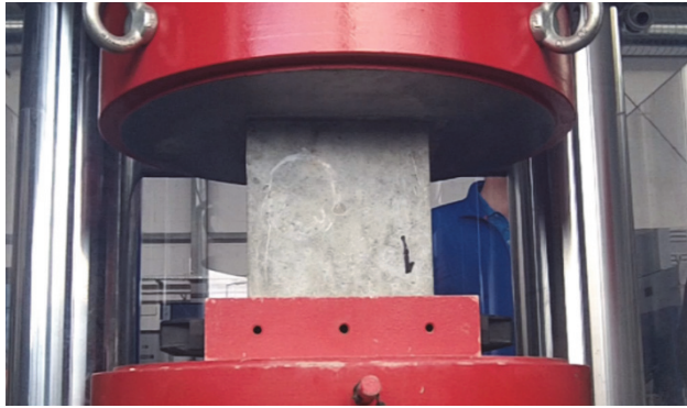
Fig. 3.2. Cube specimen prepared for compressive strength test (photo by J. Katzer)
