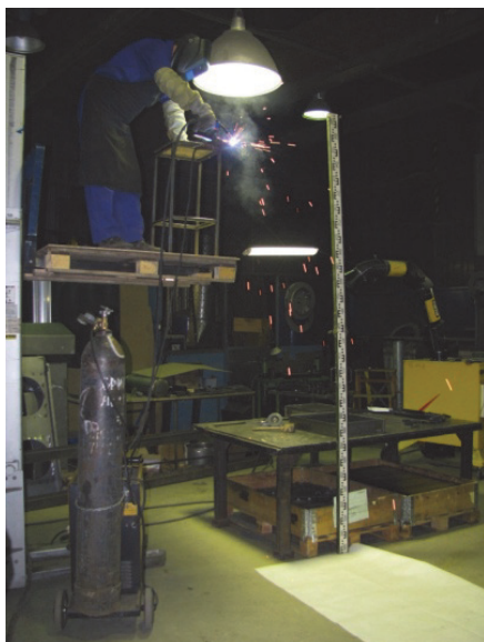
Fig. 1. Measuring the hydraulic size of the dust particles evolved while welding
