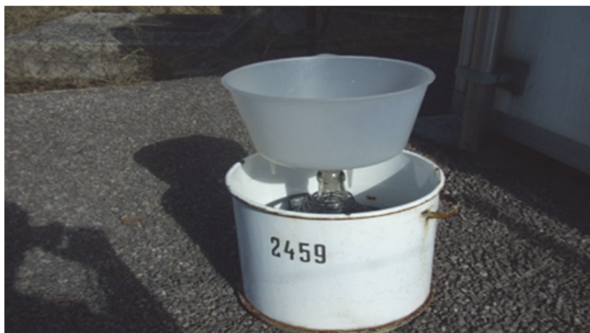
Fig. 1. Container for collecting rainfall – area AMS Oslany (Author)
