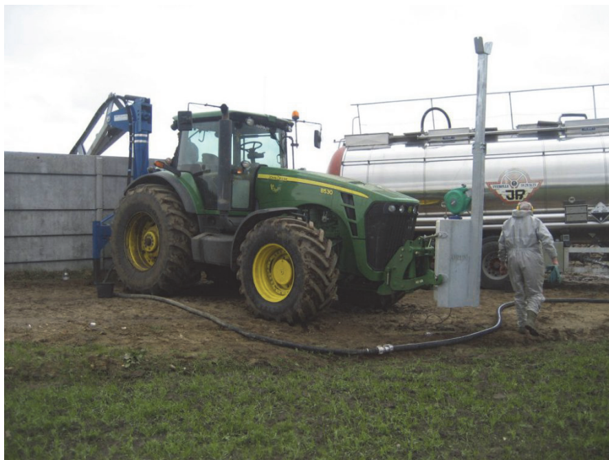
Fig. 4. Orum Smeden's "in storage" acidification system at work (Orum Smeden's)
