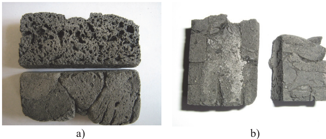
Fig. 3. Illustration of fragments of thermal insulation zones sections in complicated form structures performed by the working zone filling with fragmented elements and the subsequent heat treatment in dismountable equipment of varying complexity: a) - without limiting the free volume of formation; b) - with restriction of formation space
