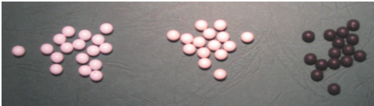
Fig. 3. The material used in the research. Spherical particles with diameter d = 6.0 \pm 0.05 mm and specific density \rho_s = 1061, 1768 and 2653 \text{kg}\cdot\text{m}^{-3}
