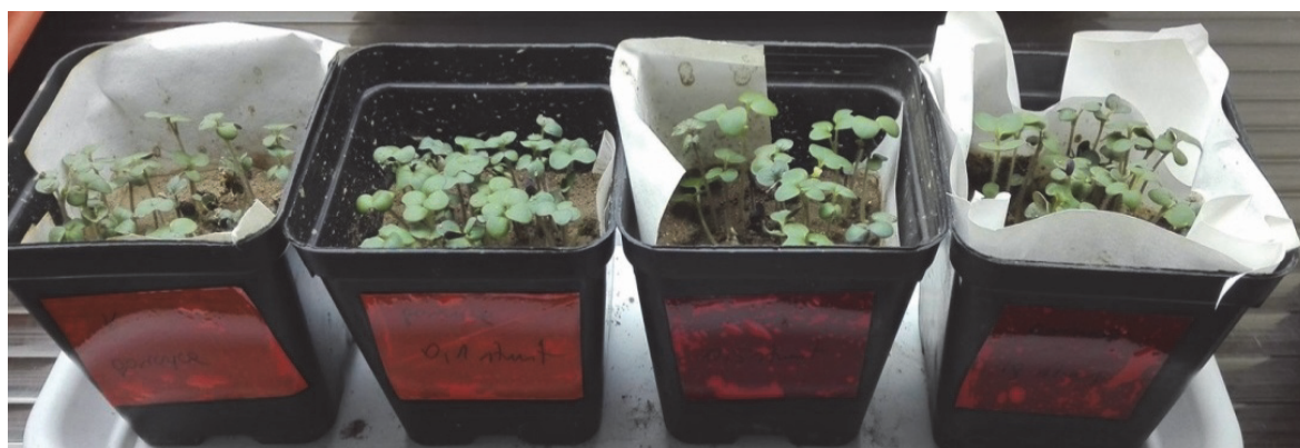
Fig. 3. Comparison of the growth of mustard after 7 days of growing: (from the left) control sample, soil with addition of 0.1 g struvite, soil with addition of 0.5 g struvite, soil with addition of 1.0 g struvite
