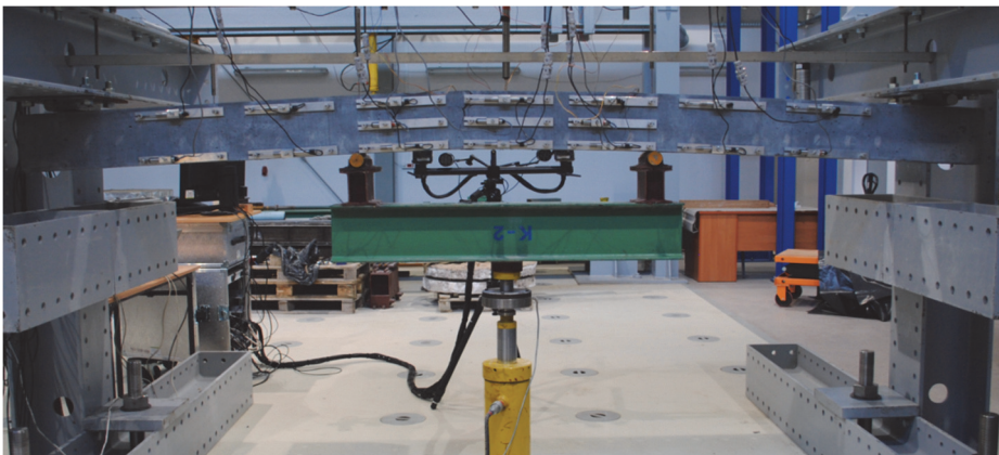
Fig. 1. Stand and static scheme of tested beams: a) schematic drawing; b) general view
