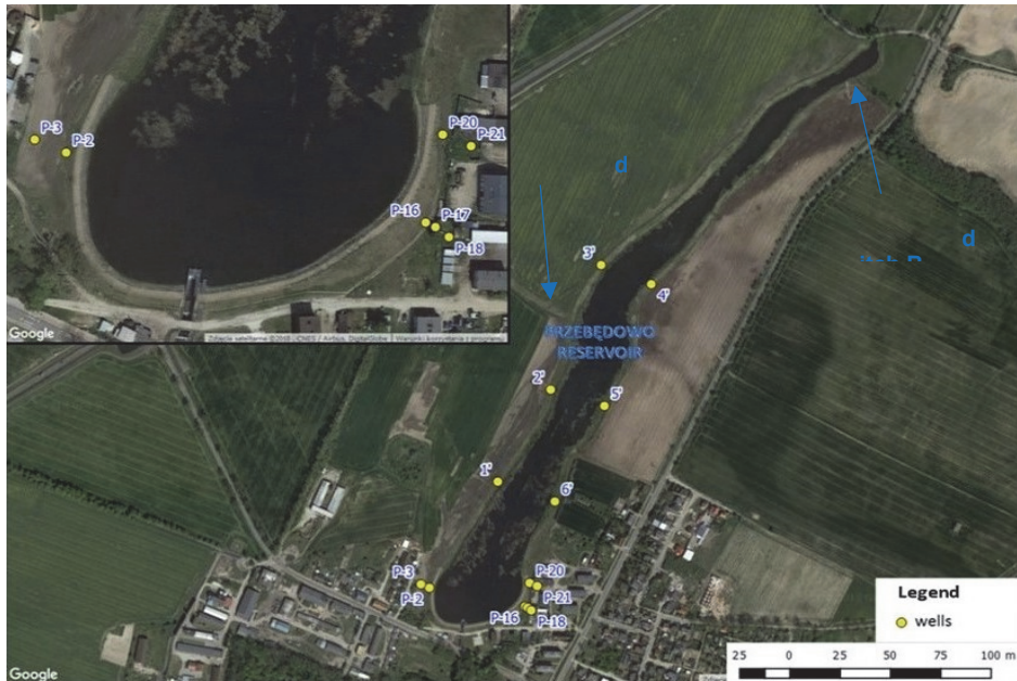
Fig. 4. Location of wells for groundwater level measurements in the area adjacent to the reservoir (source: the authors' study based on Google Earth https://www.google.pl/intl/pl/earth/ )
