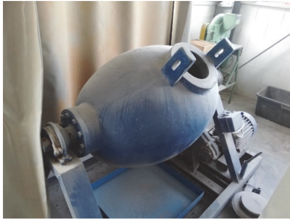
Fig. 1. Industrial grinder used for crushing lightweight aggregate granules
