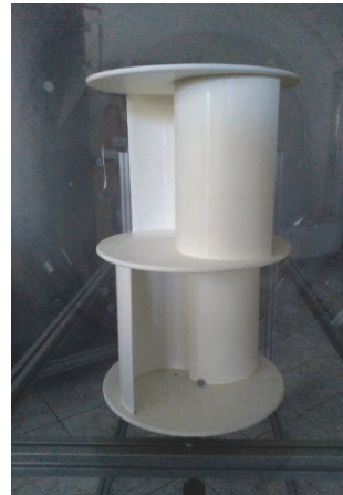
Fig. 3. View of model wind turbine rotors proposed in a hybrid system: a) Savonius, b) double Savonius
