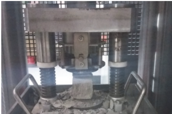
Fig. 2. Compressive strength test
