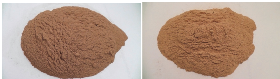
Fig. 5. Crashed and ground hazelnut shell waste (a) and walnut shell waste (b)
