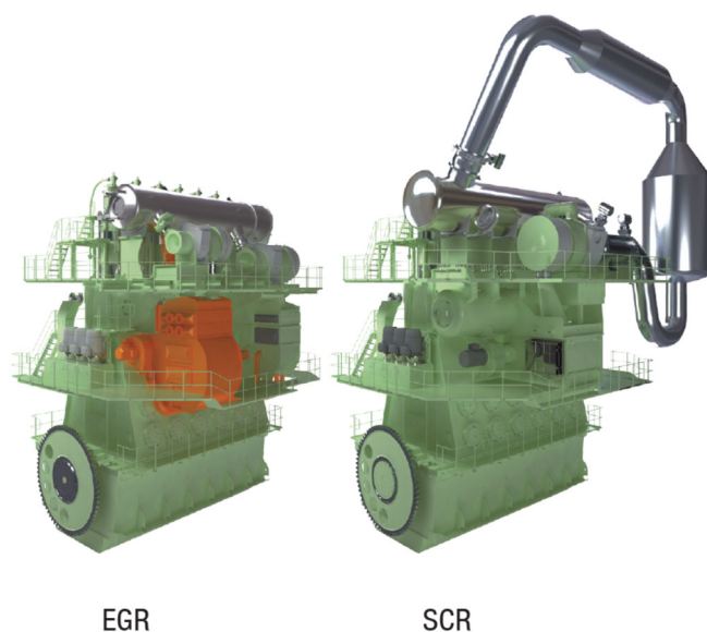
Fig. 1. Two way approach for Tier 3 engines – EGR and SCR solutions (MAN 2012)
