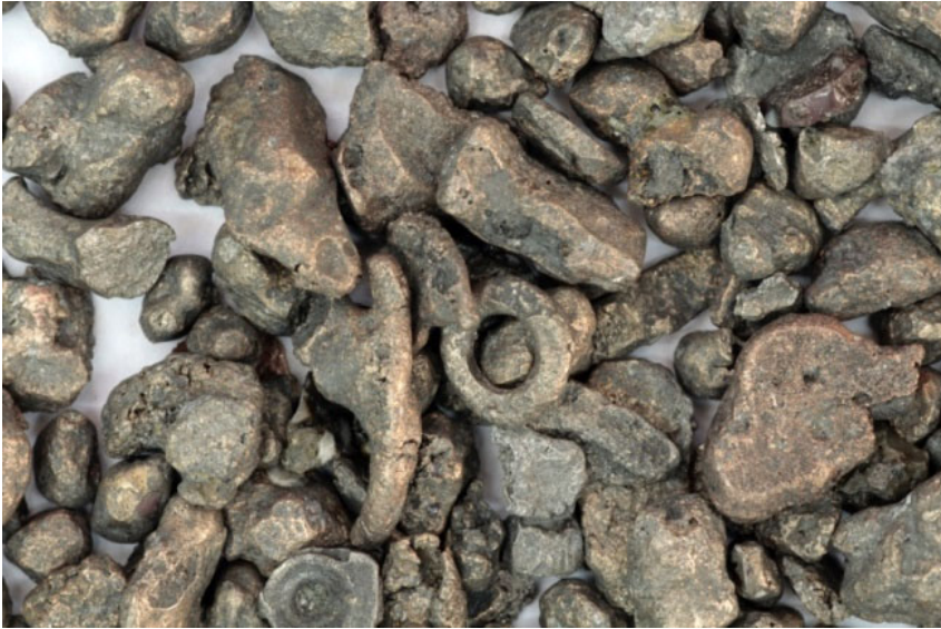
Fig. 1. Macro-photography of material rich in Cu and precious metals
