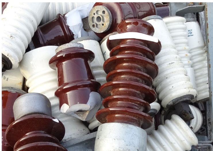
Fig. 1. Exhausted electrical insulators obtained during power line repair
