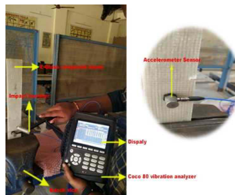
Fig. 1. Experimental analysis of E-Glass fiber beam
