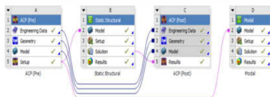
Fig. 6. Methodology for estimation of modal frequencies using ANSYS ACP
