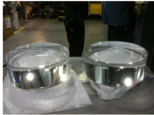
Fig. 9. Two of LIGO's 'test masses' (mirrors), so called because they 'test' (or feel for) changes in LIGO's arm-lengths caused by a passing gravitational wave. Each silica cylinder weighs 40 kg [Caltech/MIT/LIGO Lab]
