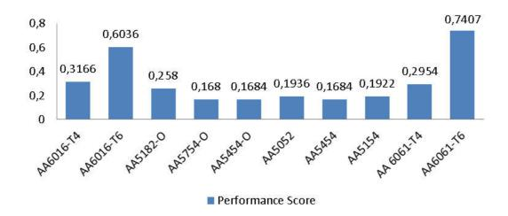
Fig. 4. Performance scores of each material according to TOPSIS
