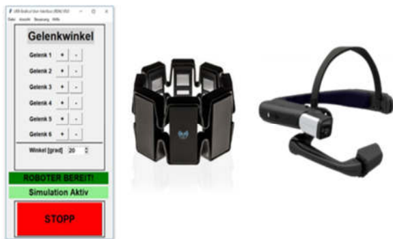
Fig. 1. Robot control peripherals; Left: Graphical User Interface; Middle: Gesture Control (Myo) [10]; Right: Voice Control (RealWear - HMT1) [11]
