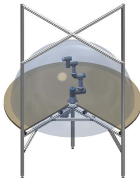
Fig. 2. CAD-Model of the multi-workstation assembly table with shown work area (light blue sphere) of the robot
