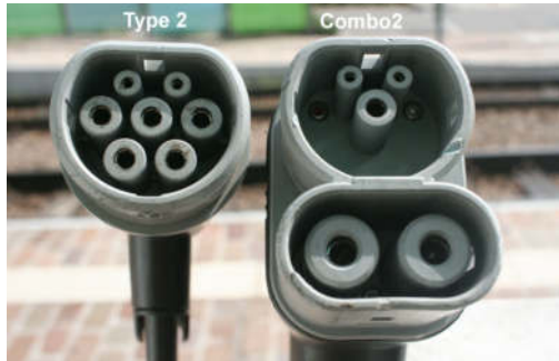
Fig. 4. Type 2 plug (on the left) next to the plug (right) Type 2 CCS / Type 2 combo / Combo 2 [18]
