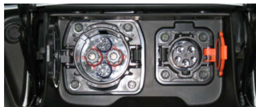
Fig. 2. CHAdeMO socket (on the left) next to the Type 1 socket (on the right) [18]
