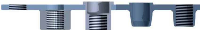
Fig. 3. Differences in threaded connections in thin-walled materials (from left): thread in material; nut welded; nitonated nut; thermally formed hole; thread in moulded material [4]
