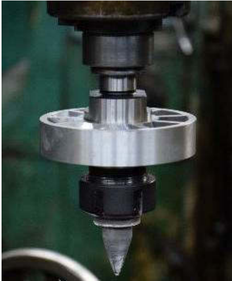
Fig. 2. Friction drilling set mounted on light milling machine AVIA FNC-25 [2]
