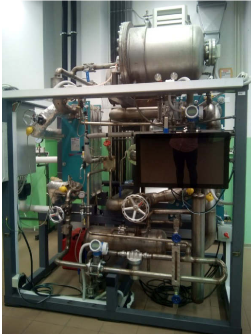
Fig. 1. ORC power plant supplied with water at 100°C (Department of Heat Engineering, West Pomeranian University of Technology in Szczecin, operating factor R227ea, 9 kW el power) [11]
