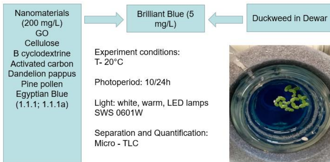
Figure 20. Detailed protocol scheme of 16 days test performed for degradation of Brilliant Blue in the presence of duckweed water plant and given nanomaterials
