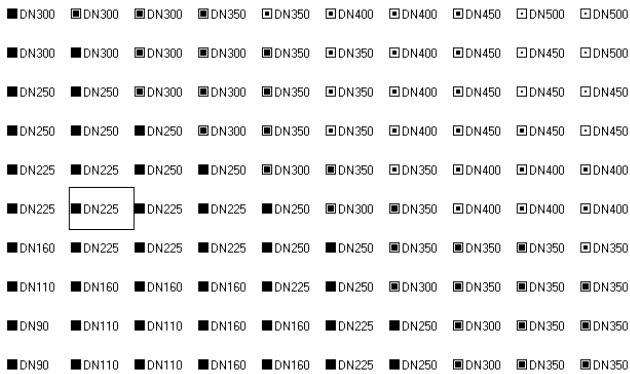
Fig. 5. An example of a topological map for the classification of pipe diameters (source: own elaboration)
