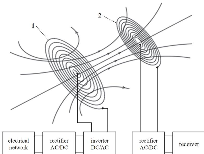
**Fig. 2.** Block diagram of the system for wireless energy transmission:
