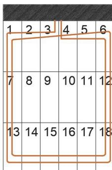
**Fig. 4.** Division of the power pad into sectors
