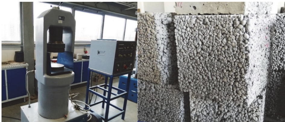
Fig. 2. The strength apparatus (left) and specimens (right) used for compressive strength and splitting tensile strength tests
