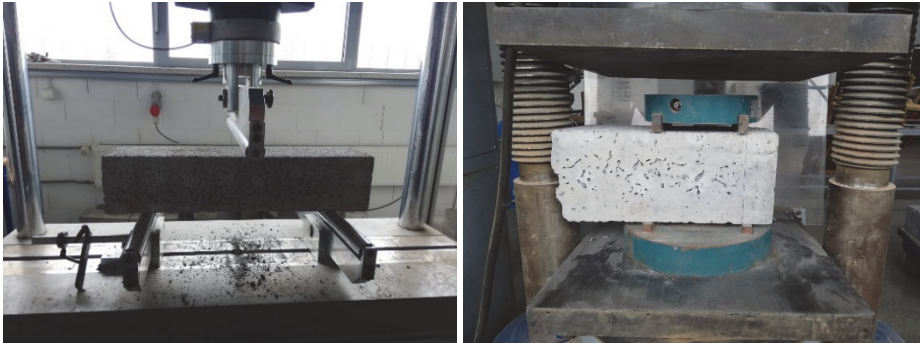
Fig. 3. Apparatus and specimen during flexural strength test (left) and shear strength test (right)
