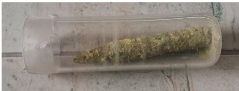
Fig. 1. Depleted uranium projectile (in a bullet shell casing) excavated in Serbia
