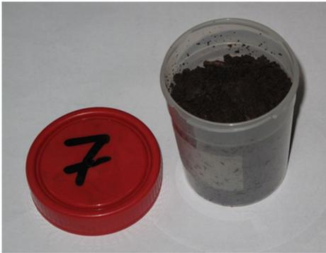
**Fig. 3.** Plastic bottle with soil sample
