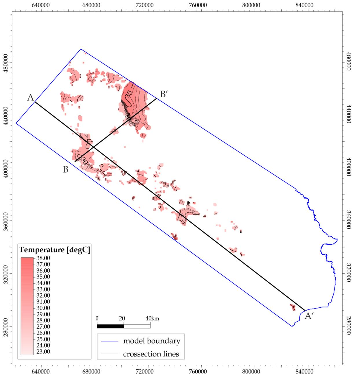
**Fig. 4.** Map of average temperatures in the 1000-1200 m below surface interval within areas of sufficient permeability. Crosssection lines marked with black lines
