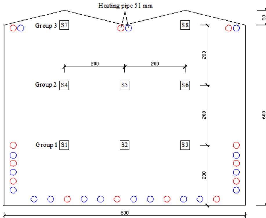
Fig. 1. Locations of sensors placed in the greenhouse
