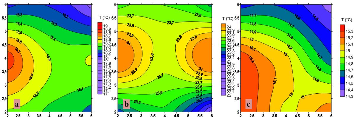
Fig. 2. The temperature distribution in the greenhouse indoor environment during the (a) daily, (b) daytime and (c) night hours
