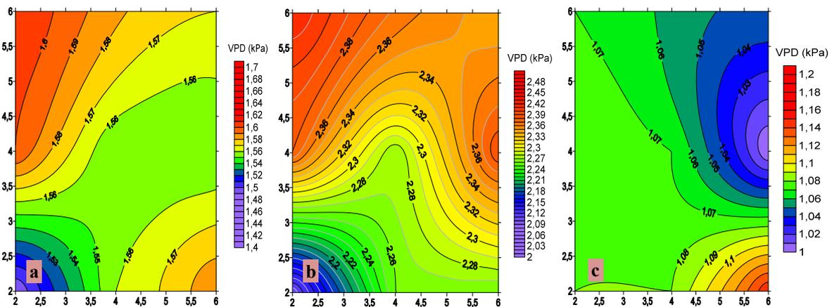
**Fig. 5.** Distribution of the vapour pressure deficit in the indoor greenhouse environment during the (a) daily, (b) daytime and (c) night hours
