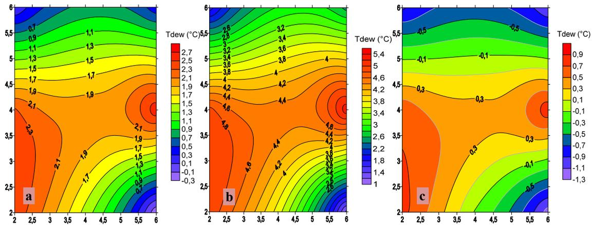
**Fig. 4.** Distribution of dew point temperature in greenhouse indoor environment during (a) daily, (b) daytime and (c) night hours
