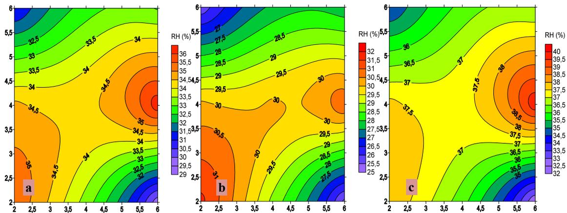
**Fig. 3.** Relative humidity distribution in the indoor environment of the greenhouse during (a) daily, (b) daytime and (c) night hours
