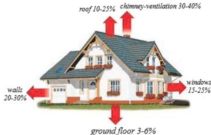
**Fig. 3.** Percentage of approximate heat loss in the house ([https://www.researchgate.net/figure/Heat-loss-in-the-building-12\\_fig1\\_331304641](https://www.researchgate.net/figure/Heat-loss-in-the-building-12_fig1_331304641))
