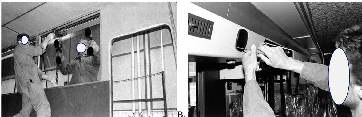
Fig. 5. A – Side windows removal; B – Removal of speaker lamps and air supply nozzles
