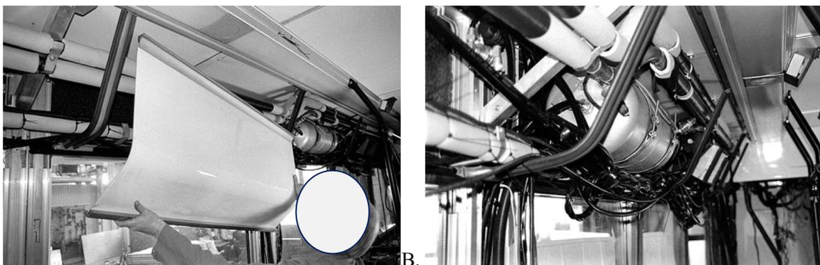
Fig. 6. A – Removal of shelf nets and flaps; B – Removal of door mechanism, air conditioning fan, air tank and electrical wires
