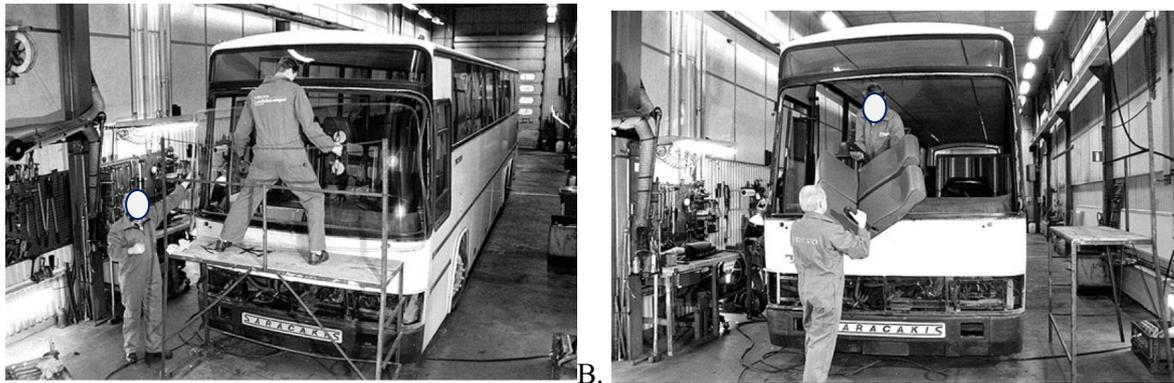
Fig. 4. A – Windshield removal; B – Seats removal
