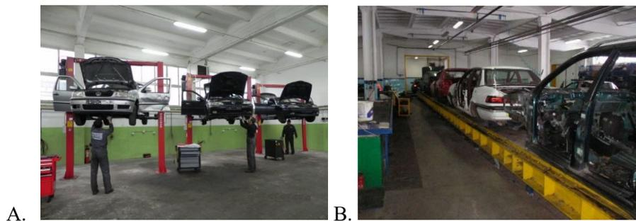
**Fig. 3.** A – lift used in cell-based dismantling; B – dismantling of components in the dismantling line
