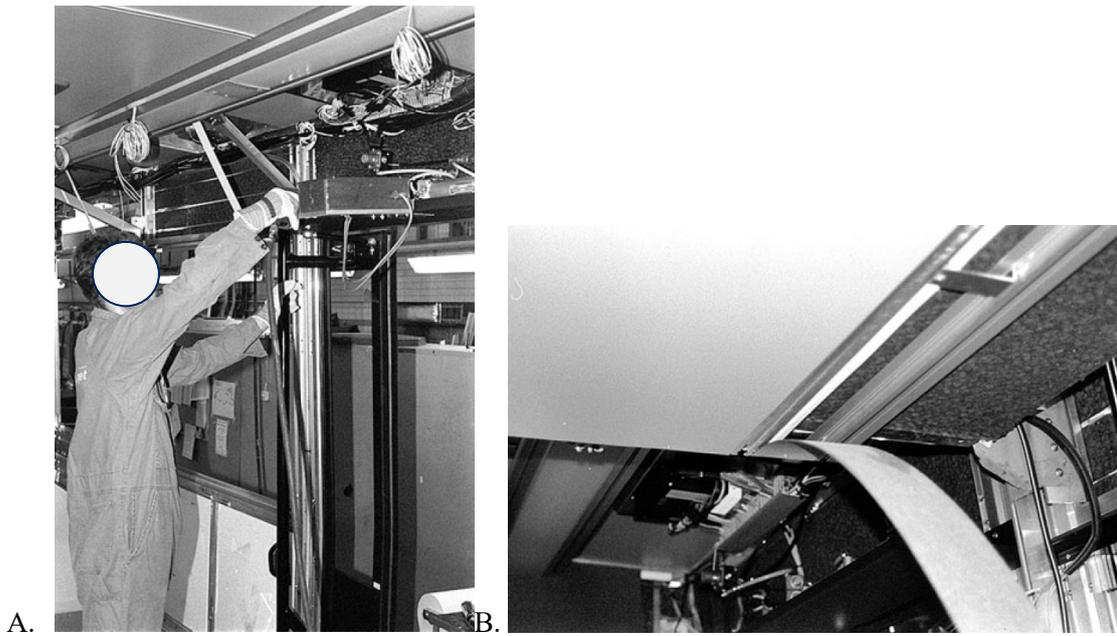
**Fig. 7.** Removal of doors and roof flaps; B – Removal of ceiling lining.
