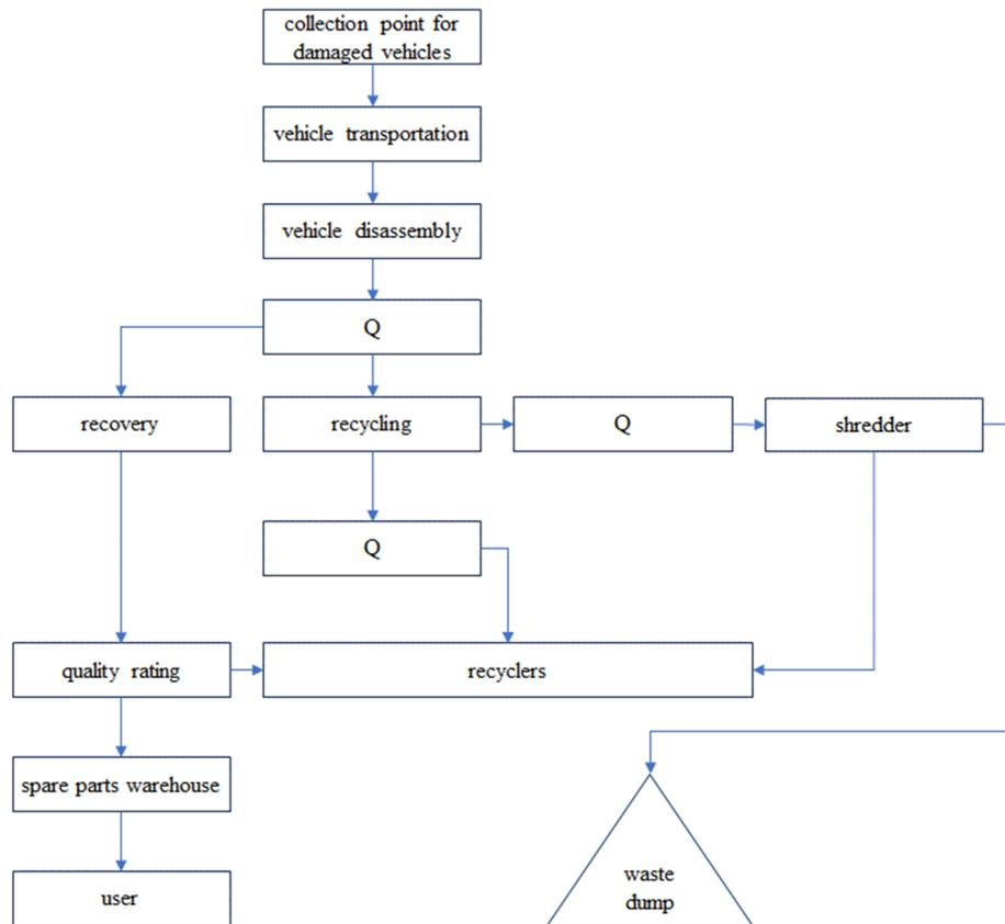
Fig. 1. Diagram of process logistics, where Q stands for pre-classification, based on (Merkisz-Guranowska 2007)
