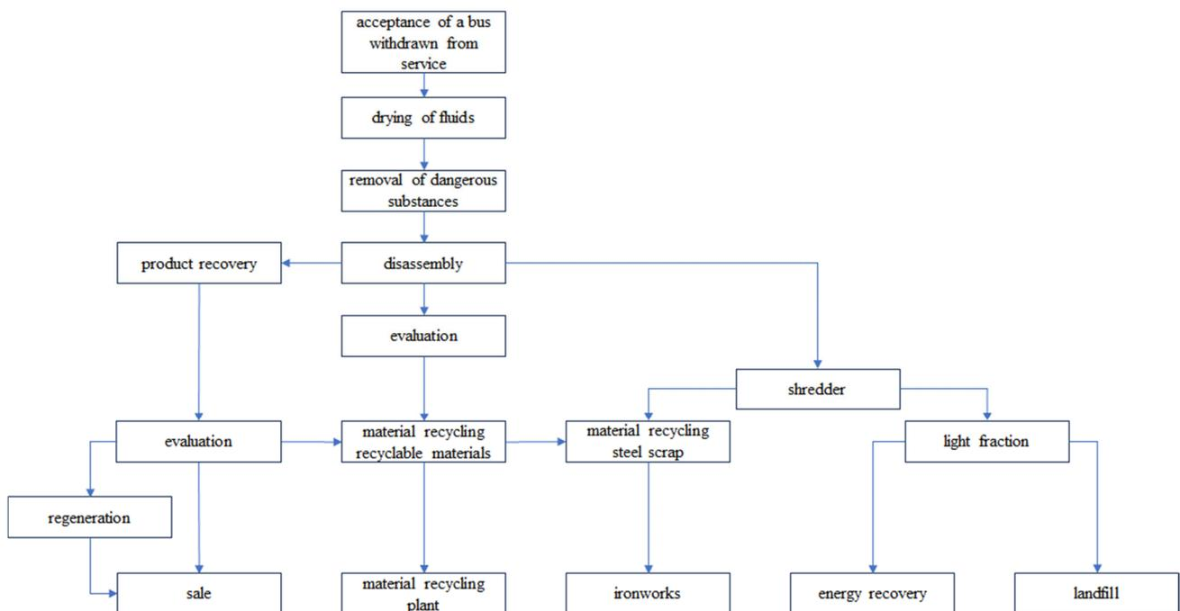
Fig. 2. General diagram of the end-of-life bus recycling process, based on (Tomczyk 2012)
