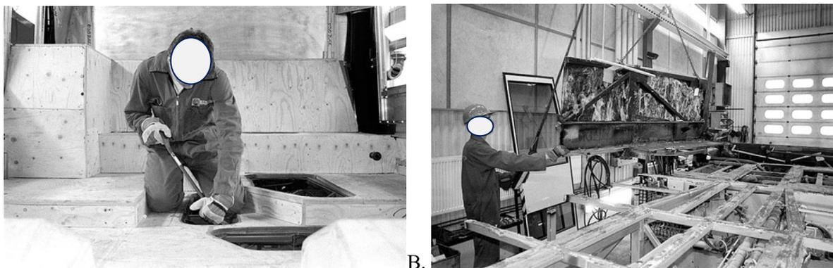
Fig. 12. A – Removal of floor slabs; B – Removal of the body sides
