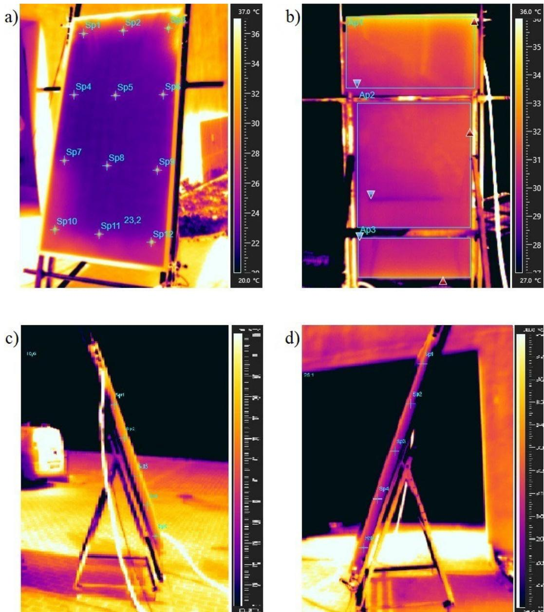
**Fig. 7.** Thermographic measurements of the collector made for a medium flow rate of 80 [kg/h] and a working medium temperature of 40 [°C]. a) front surface, b) rear surface, c) and d) side surfaces of the collector
