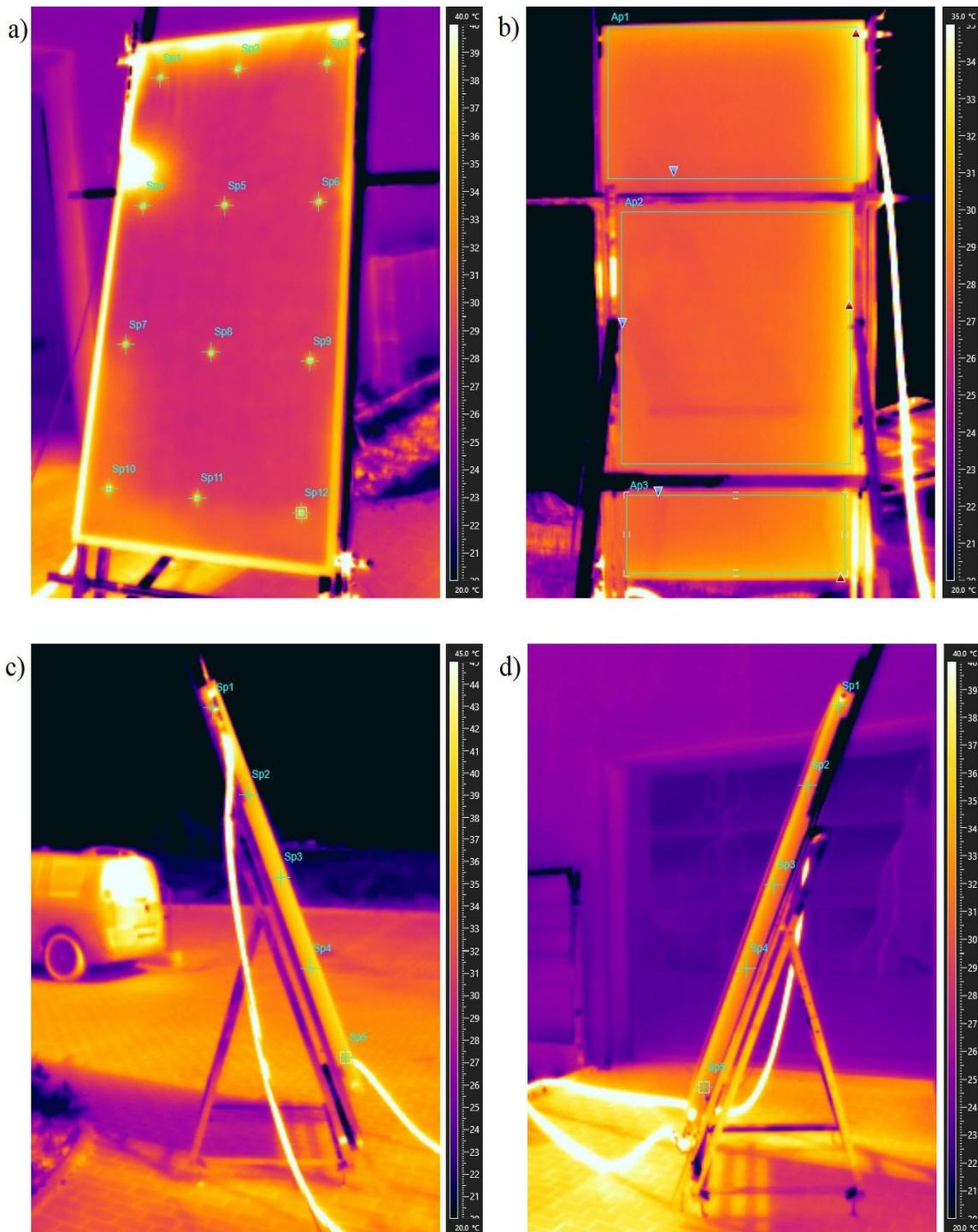
**Fig. 8.** Thermographic measurements of the collector made for a medium flow rate of 120 [kg/h] and a working medium temperature of 40 [°C]. a) front surface, b) rear surface, c) and d) side surfaces of the collector
