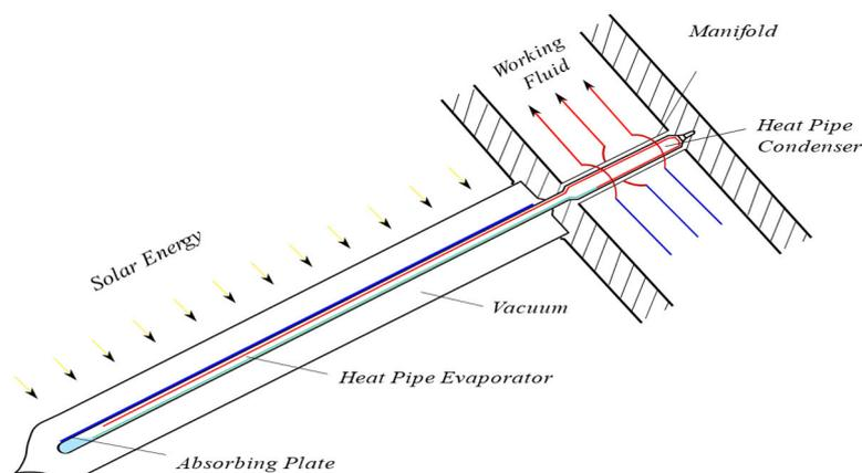
**Fig. 2.** The principle of vacuum tubes
