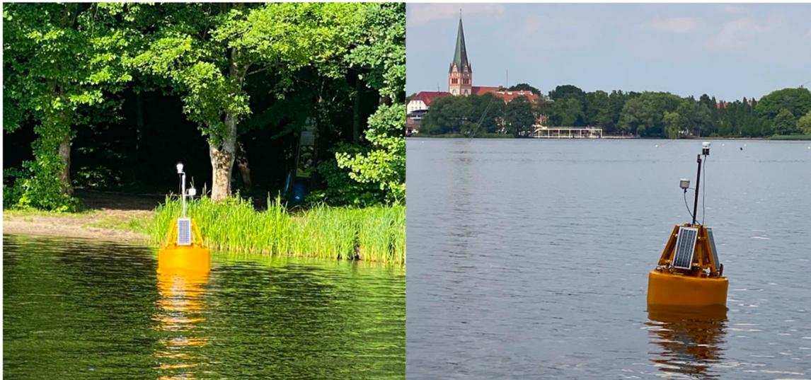
**Fig. 7.** Development version of the probe in a steel housing in the form of a full buoy during test measurements
