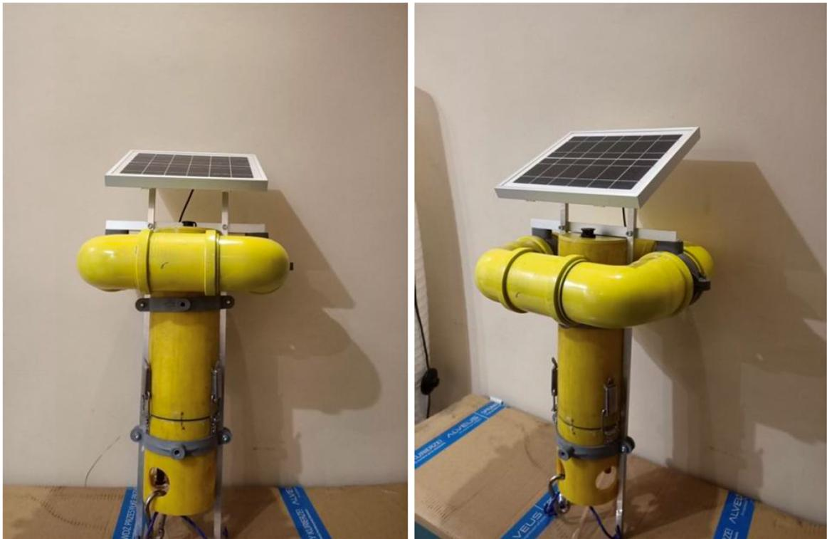
**Fig. 1.** Prototype of the measurement probe in the variant for preliminary tests
