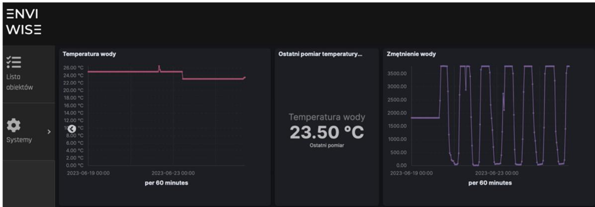
Fig. 4. Test charts of the central application dashboard – data from the temperature and water turbidity sensor
