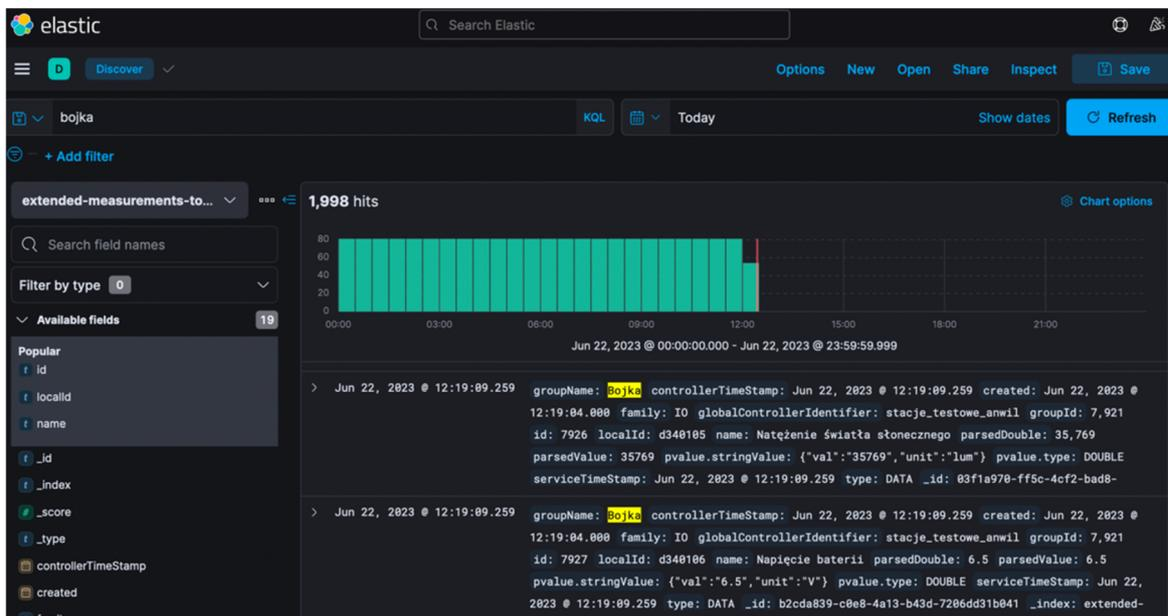
Fig. 2. Backend view of the Kafka data broker presenting test measurements from the measurement probe
